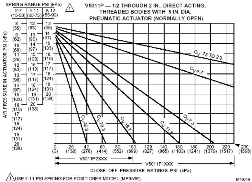
Fig. 3. Close-off ratings at various control air pressures for V5011P Valves and MP953 Pneumatic Actuators.
