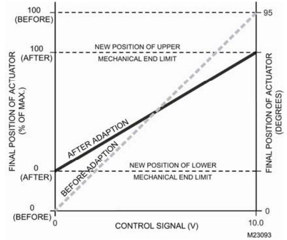
**Fig 5. Adaption (function selection switch set to 0...10 V)**
